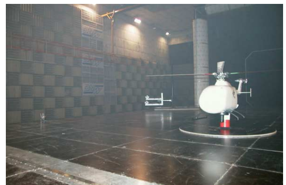
Figure 1 BO 105 model in DNW-LLF test section
