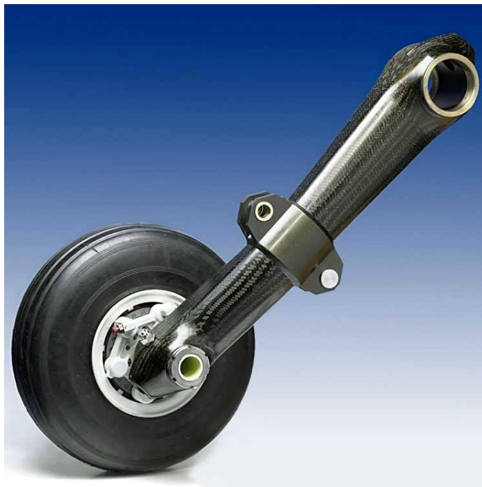
Fig. 12 Composite trailing arm NH90 helicopter (courtesy SP)
