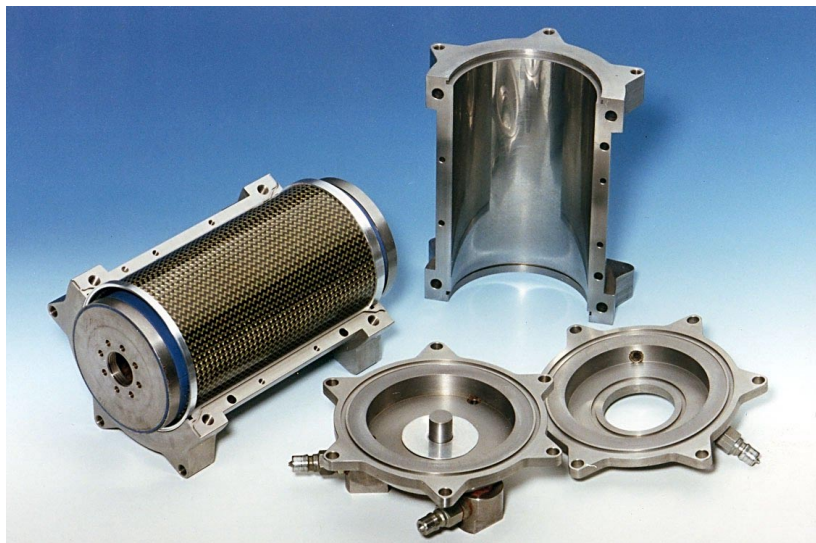
Fig. 4 Crash tube for NH90 nose landing gear and fabrication tooling
