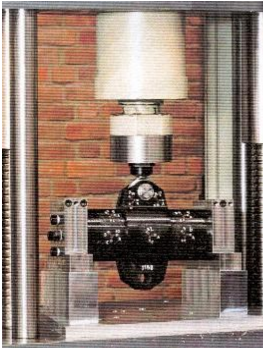
Figure 11. Test of trailing arm centre section.
