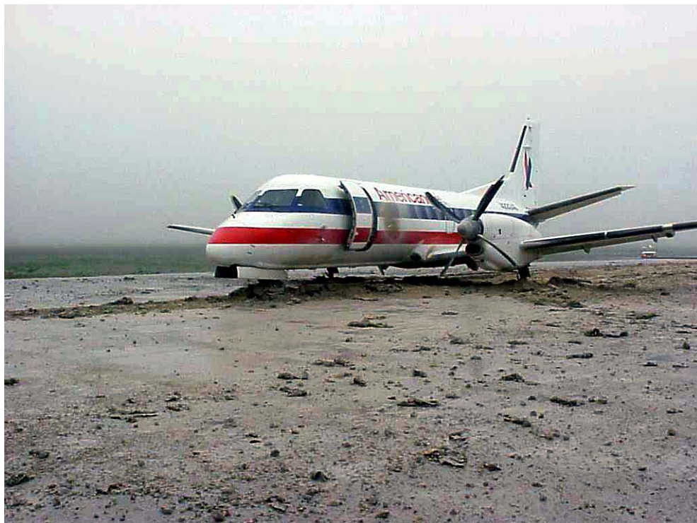
Figure 4: Overrun with a SAAB 340 that ended in a soft arrestor bed.
