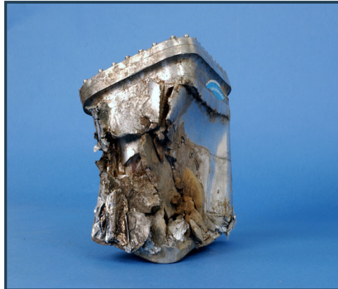
Figure 3: Heavily damaged BIOFILTER box after the accident with FOTON M1
