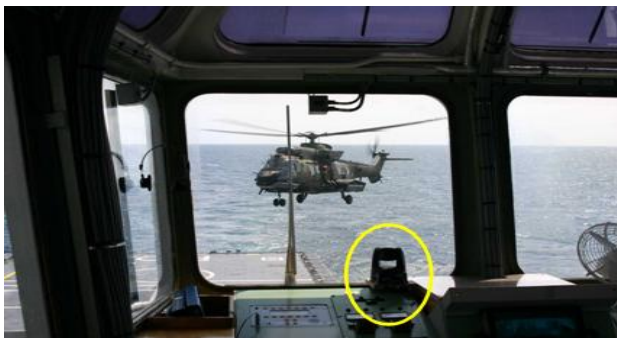
Figure 27 Video camera installed in the FLYCO cabinet.
