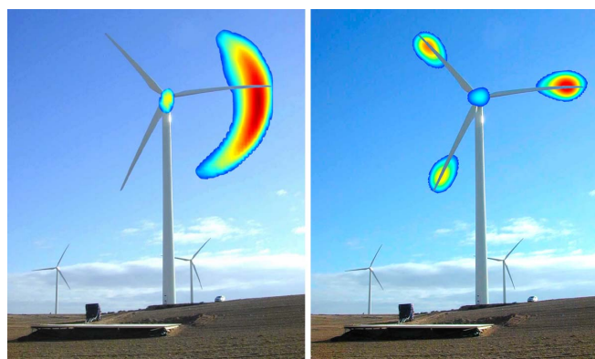
Figure 7: Wind turbine field test, post processing with stationary focus (left) and rotating focus (right).
