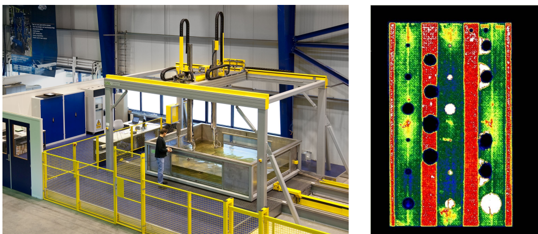
Fig. 2 Ultrasonic C-scan equipment (left) and an example of the inspection of panel NTP-B (solid laminate with 3 T-shaped stiffeners; pulse-echo inspection with monitoring of the backwall-skin reflection)
