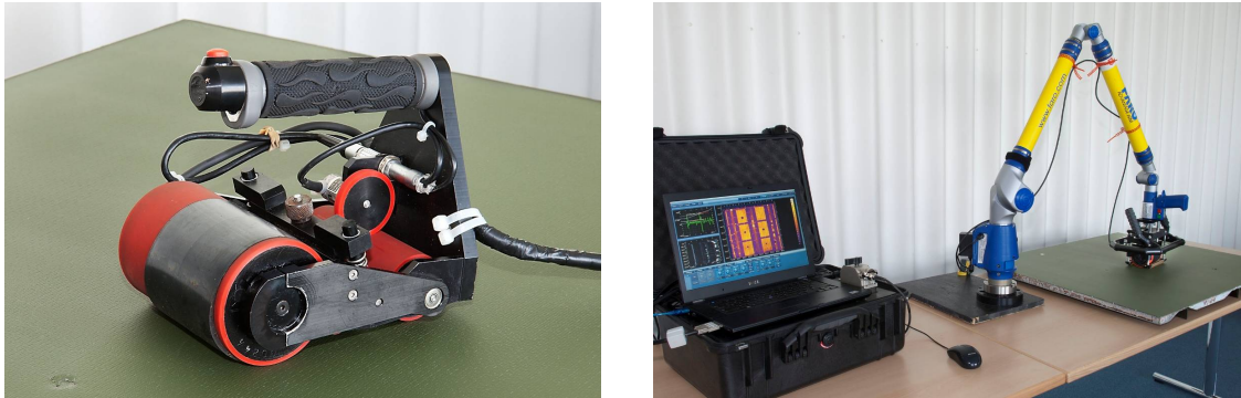
Fig. 7 UT-PA RapidScan™ with 50 mm wheel probe and 7-axis Faro scanning arm (right)
