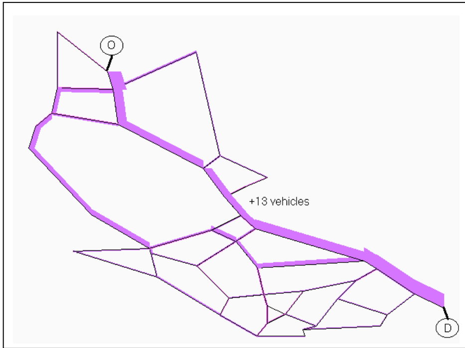
Figure 2: Diagrammatic representation of increase in arc flows following increase in an origin-destination flow (Headingley network)
