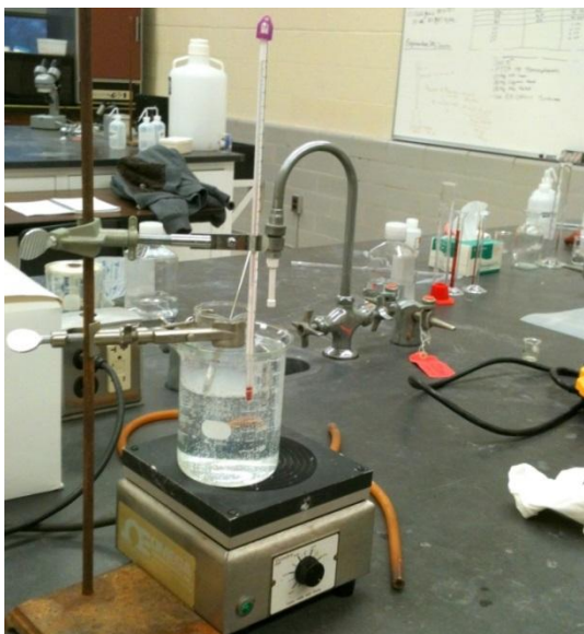
Figure 6.3: Experimental set up for PVA solution preparation
