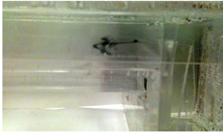
Figure 6.5: Migration multi walled carbon nanotube in 4% PVA & borax gel at 200V after 25mins
