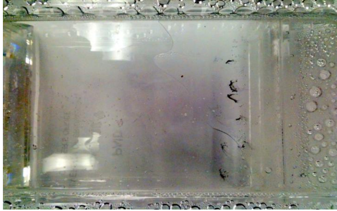
Figure 6.5: Migration multi walled carbon nanotube in 4% PVA & borax gel at 200V after 25mins
