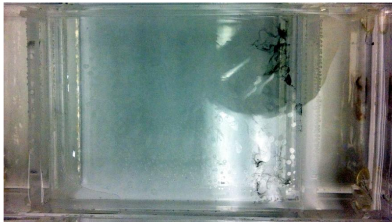
Figure 6.6: Migration multi walled carbon nanotube in 4% PVA & borax gel at 250V after 10mins
