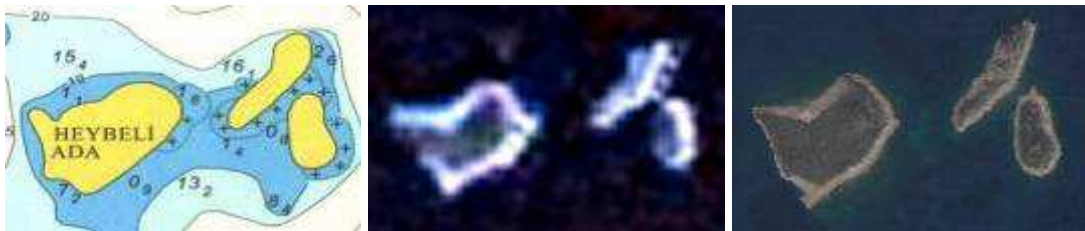
Figure 7.4. Comparison of nautical chart and Landsat GeoCover 2000/ETM+, Google Maps satellite images.
