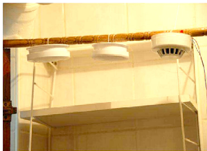
Fig. 9. Smoke sensors setup in a 4 m × 4 m small room with a ceiling height of 2.5 m.
