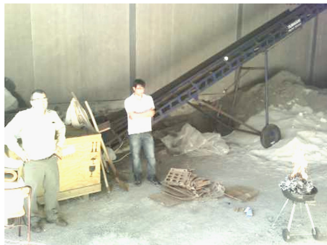
Fig. 10. The PIR sensor is in a large room of size 10 m × 12 m with a ceiling of 5 m. Cardboard is burned inside the flames.
