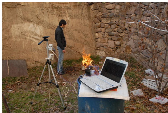
Fig. 8. The PIR sensor is encircled. The fire is close to die out completely. A man is also within the viewing range of the sensor.
