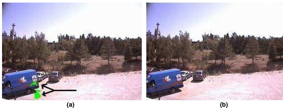
Fig. 7. (a) With the method using color and temporal variation only (Method 2) (Phillips et al., 2002), false alarms are issued for the fire colored line on the moving truck and the ground, (b) our method (Method 1) does not produce any false alarms.
