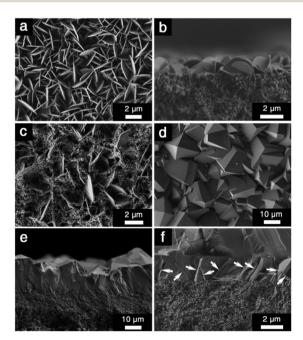
**Fig. 2** SEM images of (a, b) LDH network *in situ* grown on bare alumina substrate, (c) LDH-modified substrate dip-coated with ZIF-8 seeds, (d) the top view and (e, f) cross-sectional view of the ZIF-8 membrane. White arrows: LDH crystallites at the interface between substrate and ZIF-8 layer.
