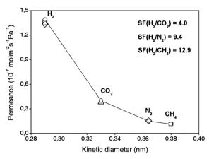
Fig. 4 Permeances of single gases ( $\bigcirc$ ) and mixed components of mixtures of H<sub>2</sub>–CO<sub>2</sub> ( $\triangle$ ), H<sub>2</sub>–N<sub>2</sub> ( $\bigcirc$ ) and H<sub>2</sub>–CH<sub>4</sub> ( $\square$ ) on the prepared ZIF-8 membrane at  $\Delta P=1$  bar and T=25 °C as a function of molecular kinetic diameters.
