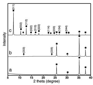
Fig. 3 XRD patterns of (a) bare  $\alpha\text{-Al}_2O_3$  substrate, (b) LDH network-modified  $\alpha\text{-Al}_2O_3$  substrate and (c) ZIF-8-LDH composite membrane. Peaks marked with dots, rhombuses and asterisks represent diffraction peaks from ZIF-8 layer, LDH network and substrate, respectively.
