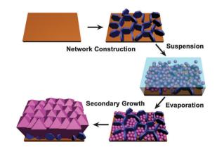
Fig. 1 Schematic illustration of the ZIF-8 membrane synthesis in the confined space of a vertically aligned layered double hydroxide (LDH) network illustrating the role of the LDH network: a "perch" for the seeds.
