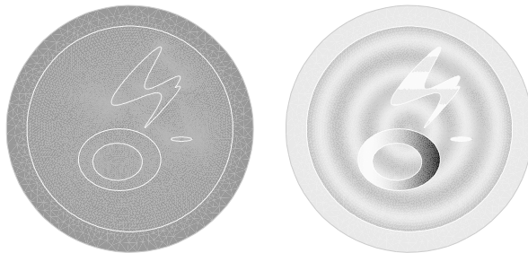
Figure 2: Perfect reconstruction test. From left to right, the initial guess, the reconstructed conductivity after three iterations
