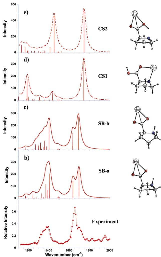
**Figure 1.** IRMPD spectrum of Pro–Na<sup>+</sup> (a). IR spectra and structures of the lowest energy Pro–Na<sup>+</sup> isomers, computed at the B3LYP/6-31G\* level (b–e).
