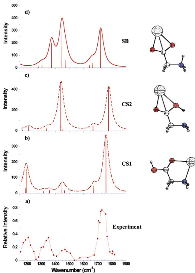
**Figure 2.** IRMPD spectrum of Gly-Na<sup>+</sup> (a). IR spectra and structures of the lowest energy Pro-Na<sup>+</sup> isomers, computed at the B3LYP/6-31G\* level (b-d).
