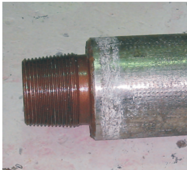
Figure 1. Description of a drillstring: a) drillstring components; b) picture of the pin part of a tool-joint.
