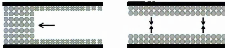
Figure 5.13 The schematic mechanism of desorption (a) and adsorption (b) processes. Circles represent mobile water molecules, crosses are immobile, surface water molecules.
