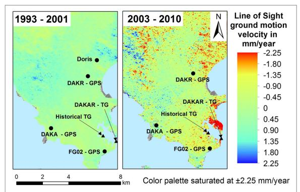
**Figure 6.** Line of Sight ground motion velocity in mm year<sup>-1</sup> for 1993–2001 (ERS 1–2 data, left) and 2003–2010 (Envisat data, right). For figure readability, the color palette is saturated at its extreme values.
