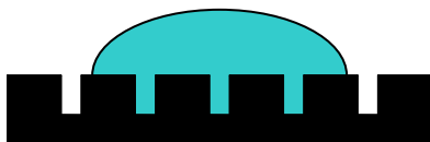
Figure 17 – Schematic diagram showing a droplet of water on a patterned surface giving rise to the Wenzel wetting regime.
