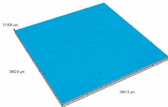
Figure 2 – Continuous axonometric image for the non-irradiated reference sample after ultrasonic cleaning.
