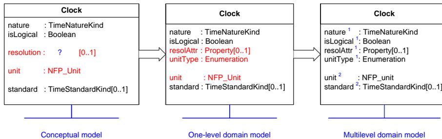
Fig. 5. A multilevel model for MARTE clocks.
