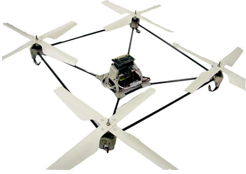
Fig. 1. The X4-flyer UAV
