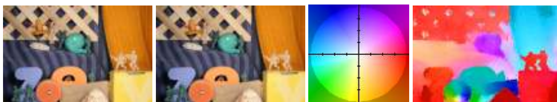
Figure 2.3: Two frames and color code for representing the flow field direction from an optical flow benchmark [BRS + 07], estimated optical flow with our method presented in chapter 7. Challenging problem: non smooth field, diverging fields ...
