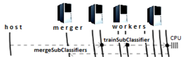
Figure 5. Parallelization of a random forest training. Each subClassifier/small forest is trained over the detected CPU cores through the Weka library (replacing classifier training in Figure 2 part III step 2)
