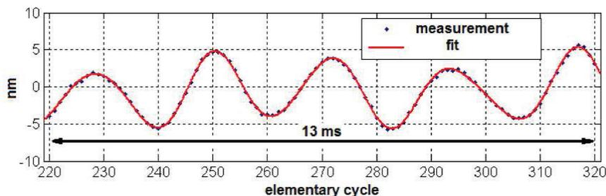
Figure 4.: One hundred successive length measurements (an offset of  $\approx 7.5$  m is subtracted, for clarity). One point corresponds to one  $A1 \Rightarrow A2 \Rightarrow A3$  sequence (one “elementary measurement cycle”). The red curve is a fit obtained using 8 harmonic (sine) functions.
