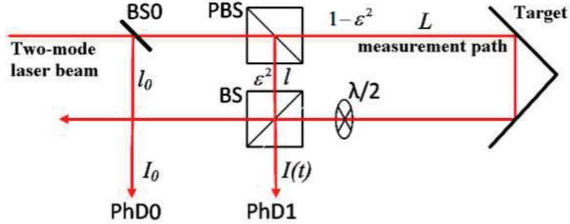
Figure 1.: Schematic diagram of the telemeter. BSO: beam splitter plate; (P)BS: (polarizing) beam splitter cube.
