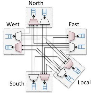
Fig. 4. Structure of a DSPIN NoC router
