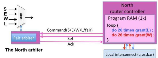
Fig. 5. Programmed arbitration in a NoC router multiplexer
