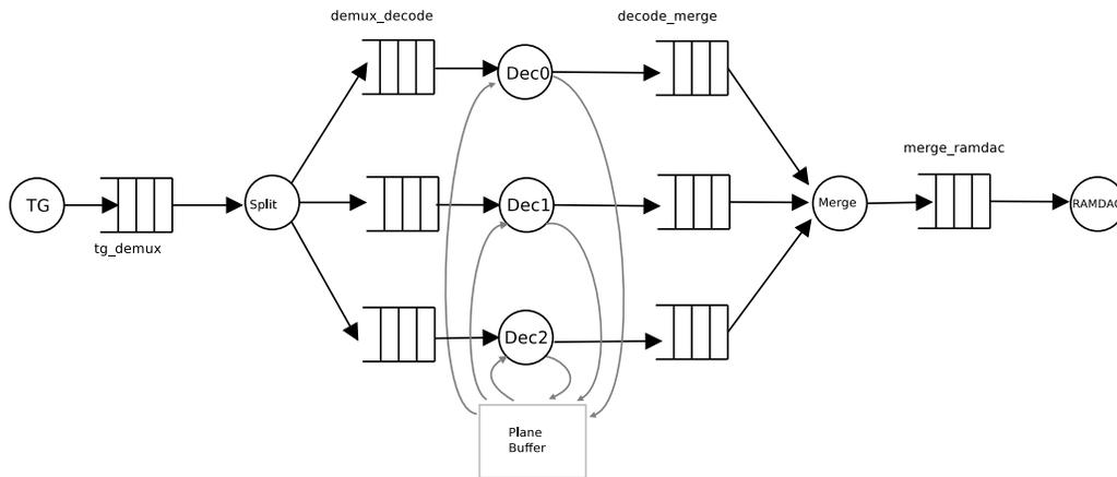
Fig. 7. Task and Communication Graph of parallel H.264
