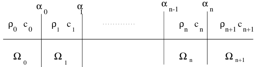
FIGURE 1. Cracks \alpha_k separating elastic media \Omega_k and \Omega_{k+1} . The physical parameters are the density \rho_k and the sound speed c_k .
