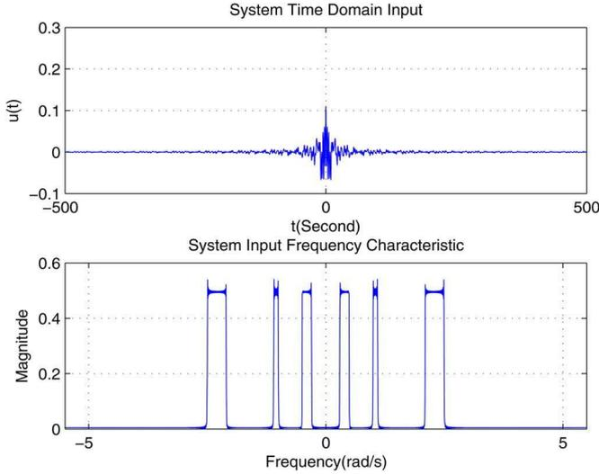
Fig. 5. Input signal in the time and frequency domain of the Hammerstein model.
