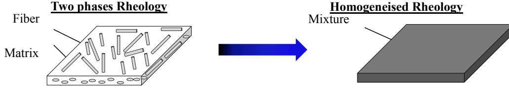
FIGURE 1. Fibre reinforced composites mainly described by two phases are described here as a homogeneous mixture characterized by its fiber fraction f . All the parameters and variables here described represents the mixture of both phases.
