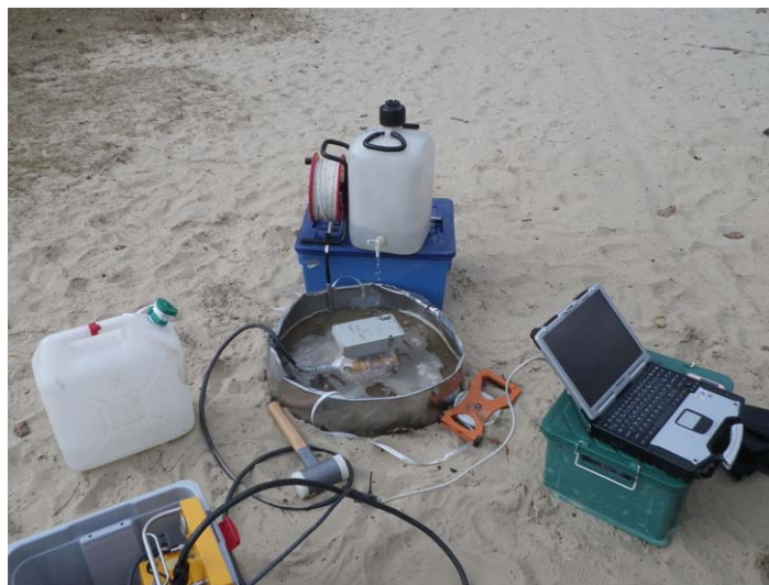
Figure 2. Picture of the experiment. Ring infiltrometer filled with 5 cm of water, the 1.6 GHz antennae are in the middle protected from water by a plastic cover. We used a water level controller coupled with a tap-tank to maintain the 5 cm of water.
