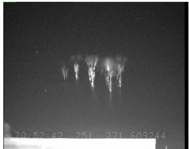
Figure 4. A frame (20 ms) displaying a carrot sprite event recorded on 17 November 2006 at 20:52:42 UT. The location of this event is given in Figure 2. The characteristics of the parent lightning stroke are given in the last line in Table 1.
