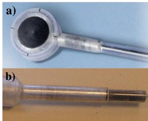
figure III.10_a) chambre plate de type NACP (IBA Dosimetry) ; b) chambre cylindrique de type Farmer, NE2571 (NE Technology)
