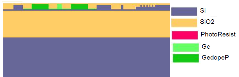
Figure 148: Definition of the intrinsic Ge core of the modulator with side contacts
