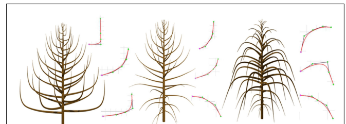
FIGURE 7 | Examples of structures whose branches shapes are defined as interpolation of three curves (shown on the right of each tree). Lengths of lateral branches are also dependant of the position of the branches on the trunk and is controlled with an extra graphical function.
