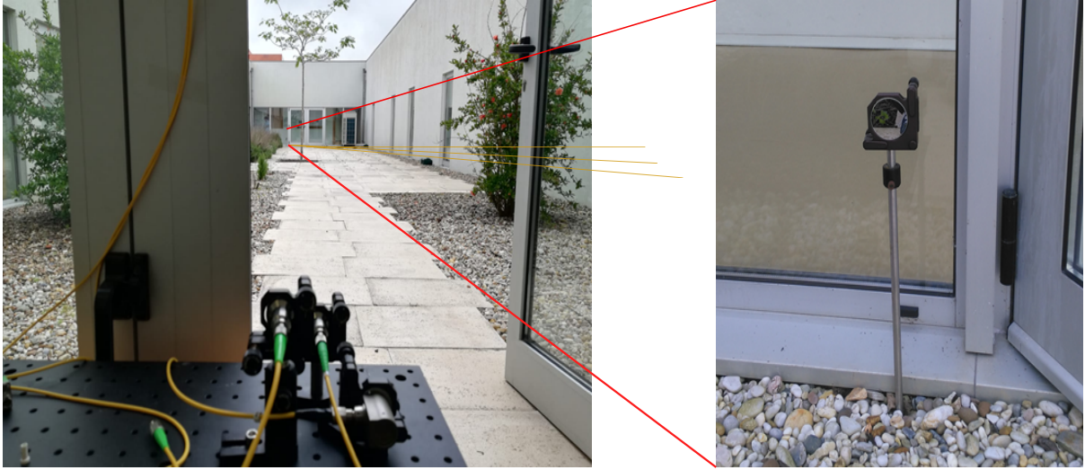
Figure 5.3: Snapshot of the FSO devices consisting of two fiber collimators and a two-inch mirror.
