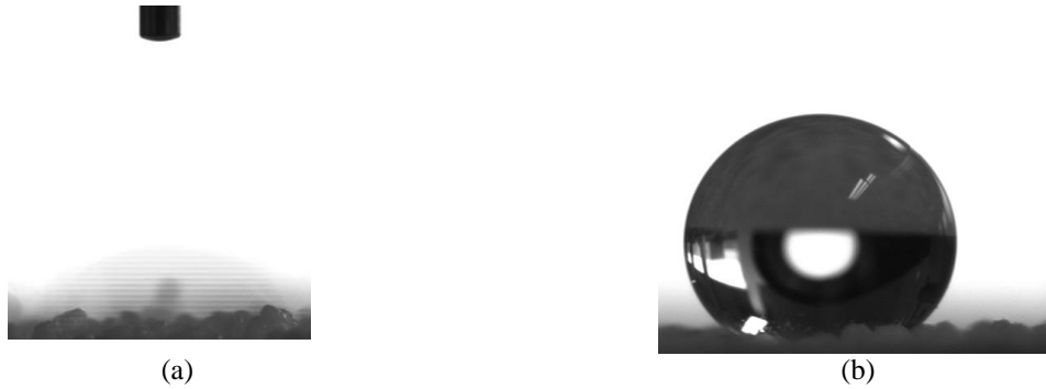
Fig. IV. 18 Snapshots of the angle of contacts (a) raw Suglets (b) coated particle with 1000 rpm and 60 s treatment.
