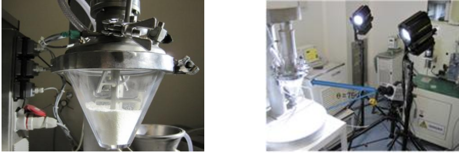
Fig. II. 13 The installation of the apparatus (a) transparent vessel, (b) high speed camera.
