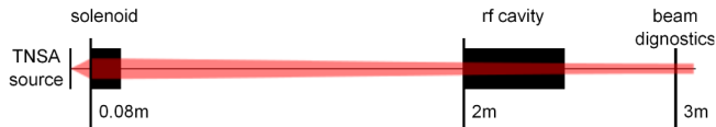
FIG. 1. The 15 cm long pulsed solenoid is positioned 8 cm behind the laser target and is typically set to focus 9.6 MeV protons at 3 m (maximum field at the solenoid of 7.5 T). The cavity (550 mm long) starts at 2 m and is followed by a diagnostic box around 3 m, where RCF stacks, a diamond ToF detector and a magnetic dipole detector can be placed (details in text).
