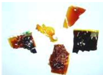
Fig. 1: Polyepoxy foils exposed to 11.1 MeV/u U ions ( 2 \times 10^{11} ions/cm 2 ) suffer from extreme radiation damage including graphitisation and embrittlement.
