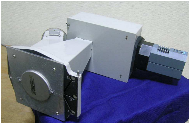
Figure 1: Photograph of the readily assembled prototype gamma imaging system showing the ANDOR CCD system (right), being coupled at 90° using an optical system, to a CsI screen (front).
