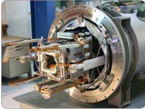
Figure 2: Straight SIS100 prototype dipole magnet manufactured at BNG.
