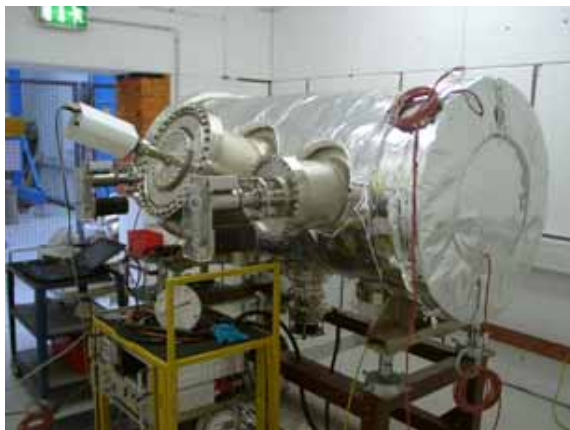
Figure 4: HV test of the new 300 kV electrostatic septum.
