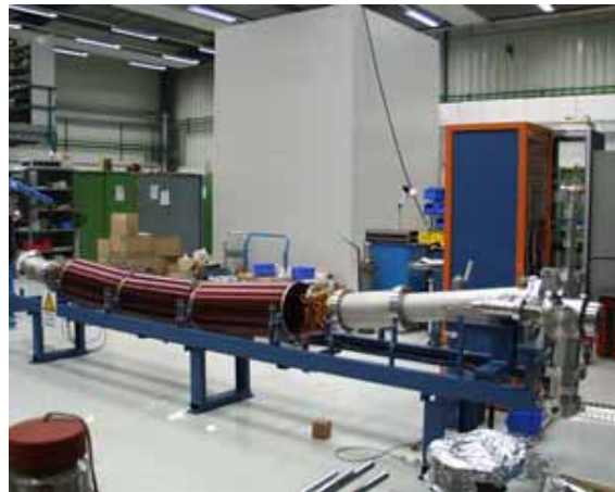
Figure 3: NEG coating of a dipole chamber at GSI
