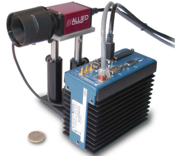
Figure 2: National Instruments Compact Vision System & attached Firewire CCD camera and remote controlled iris.
