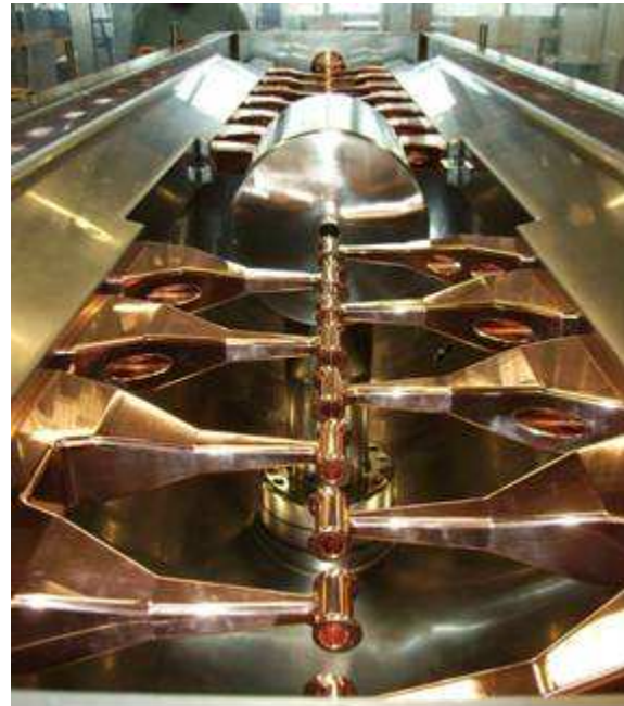
Figure 2: Picture of the IH-structure cavity, prepared for rf-measurements.
