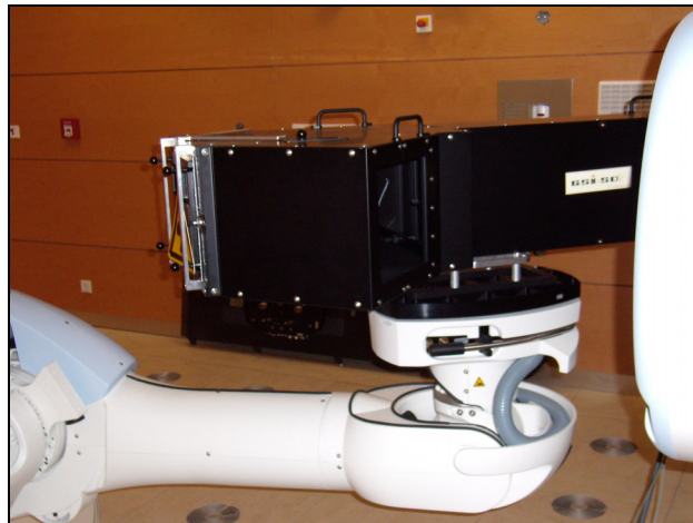
Figure 3: Robot arm with isocenter-diagnostics at the patient position in front of the beam nozzle (at right)
