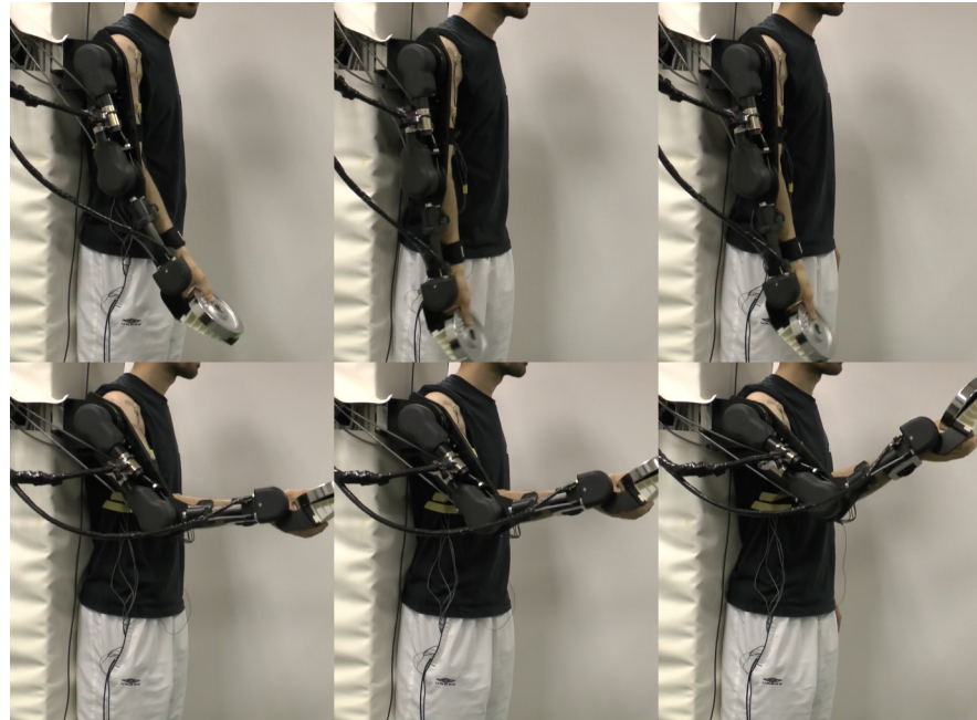
Fig 8. Sequence of photographs taken during the experiment that illustrate the state of the exoskeleton at the end of the 3 stages. Images in the first sub-row show the end-effector when it moved the object to the lower reference position, while the images in second sub-row show it in the upper position.
