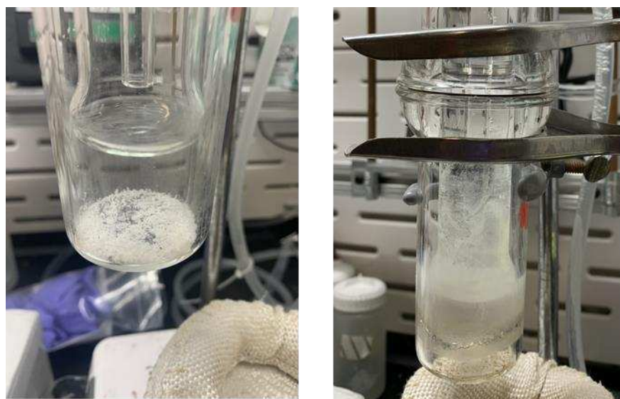
Figure S5.37. Photos of nylon 4/6 (275 mg) before and after recycling by chemolysis with \text{ZnCl}_2 at 290 \text{ }^\circ\text{C} (external temperature), 18h.
