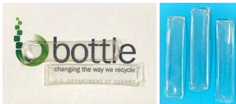
Figure 5.12. Photographs of thin films of nylon 4/6- co -nylon 4 in ~50/50 composition.
