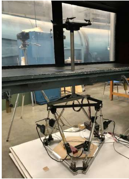
Figure 2.3: DJI Phantom 3 wind tunnel test bed at Old Dominion University [7]
