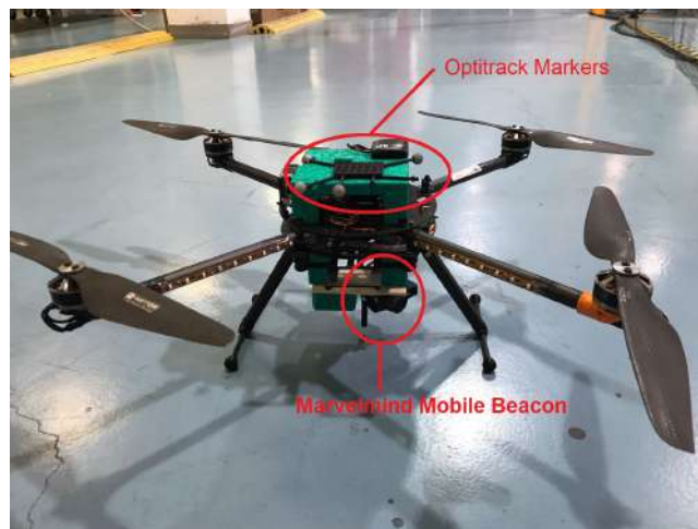
Figure D.10: UAS with Marvelmind beacon and optical marker for motion tracking
