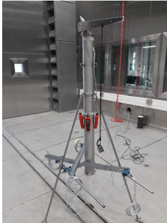
Figure 4.3: F/T sensor calibration with check loads
