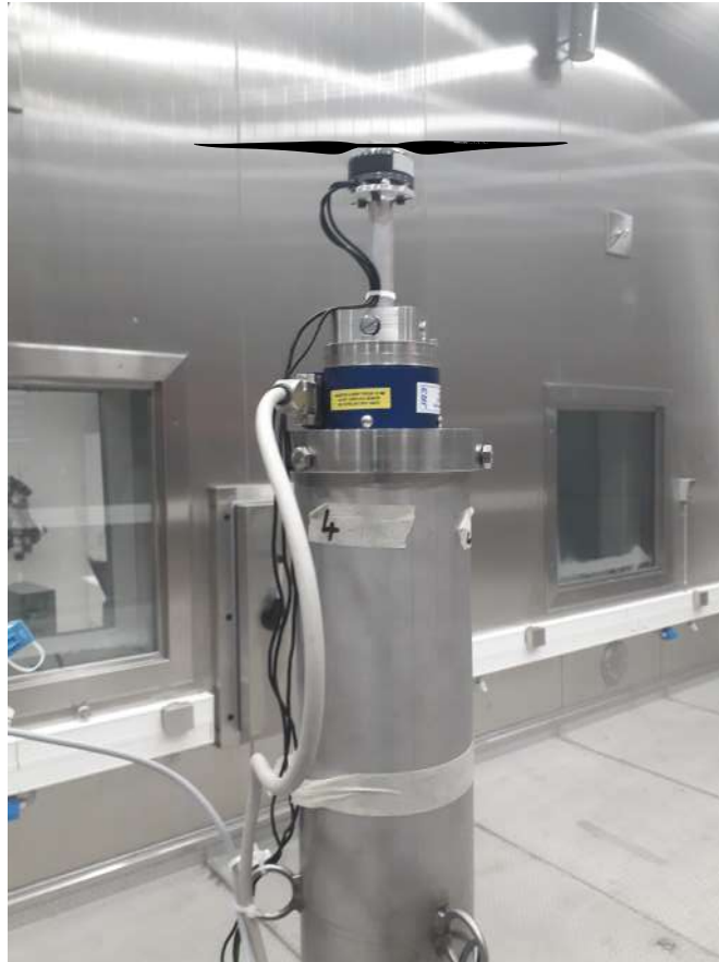
Figure 4.7: Propeller testing - setup details
