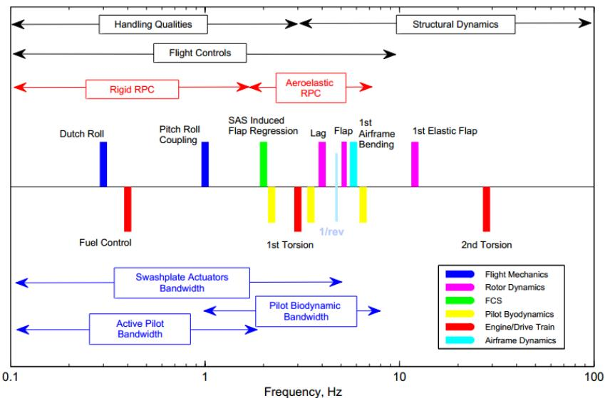
**Figure 1-8. Characteristic frequencies<sup>5</sup> of conventional helicopter dynamics, from (Serafini, 2008)**
