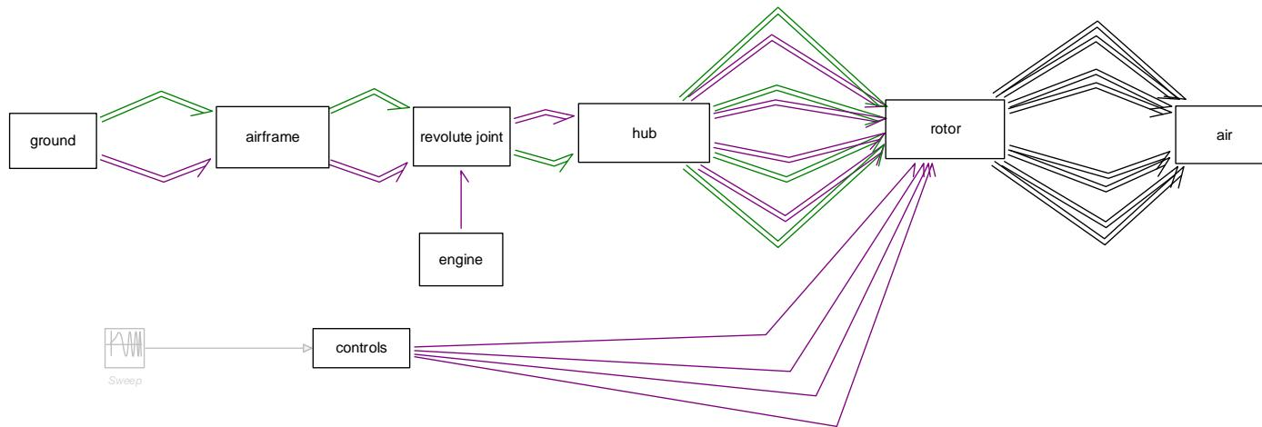
**Figure 2-15. Rotorcraft system model using bond graphs**
