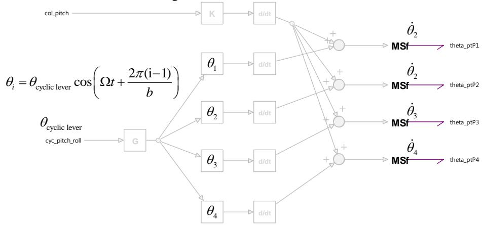
**Figure 2-14. Controls subsystem**
