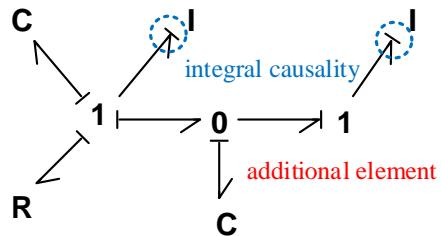
**Fig. 10.** Taking into account the elasticity between the two masses
