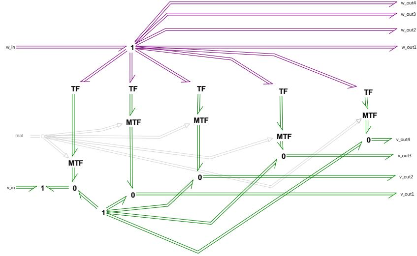
**Figure 2-13. Hub subsystem and power outputs to blades**
