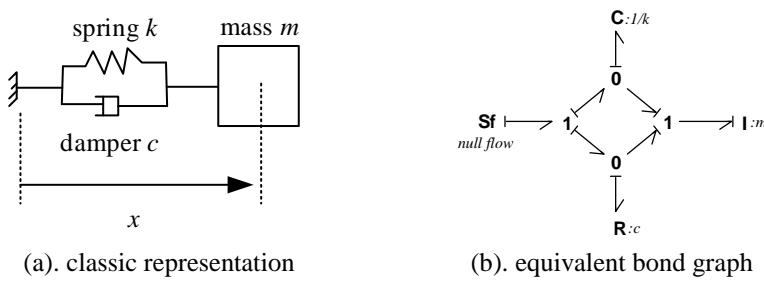
**Fig. 5. Spring-damper mass system**
