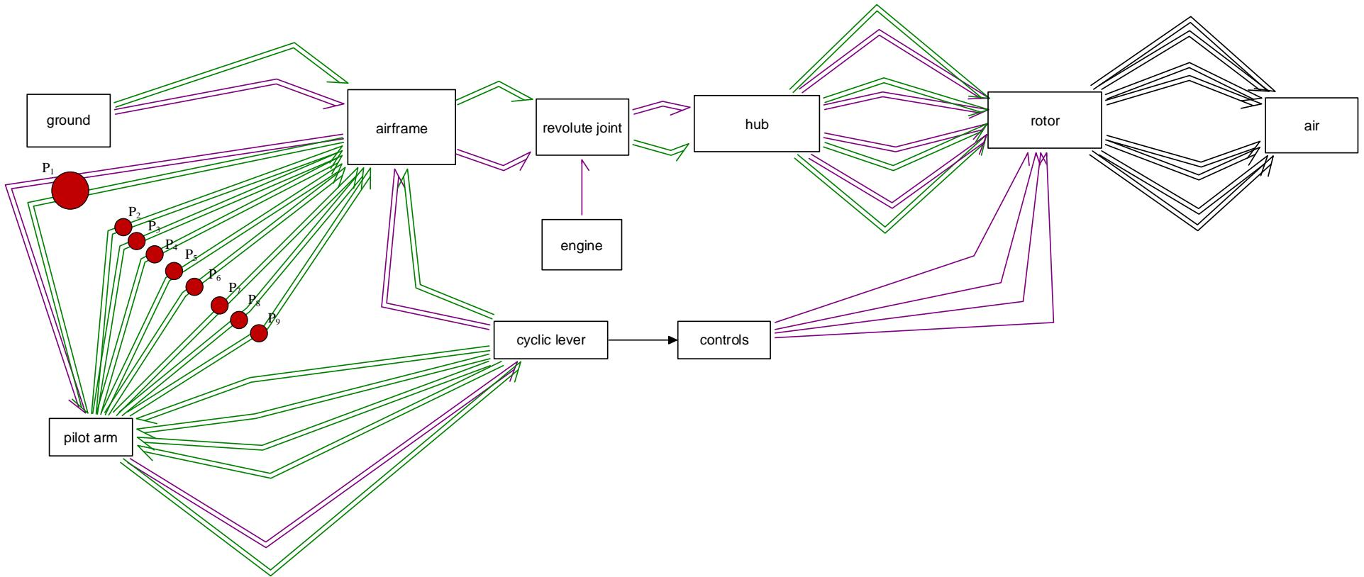
**Figure 4-2. Rotorcraft bioaeroelastic system model using bond graphs**
