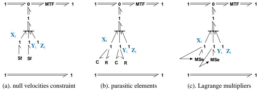
**Figure 2-7. Three methods to implement joint constraints**
