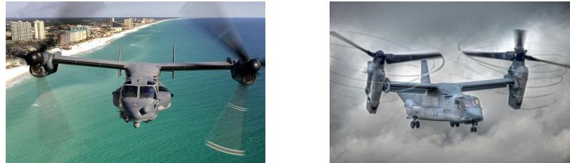
**Figure 1-1. Tiltrotor Boeing-Bell V-22 in airplane and helicopter mode**
