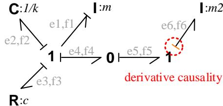
**Fig. 9. Simplified two mass system bond graph**
