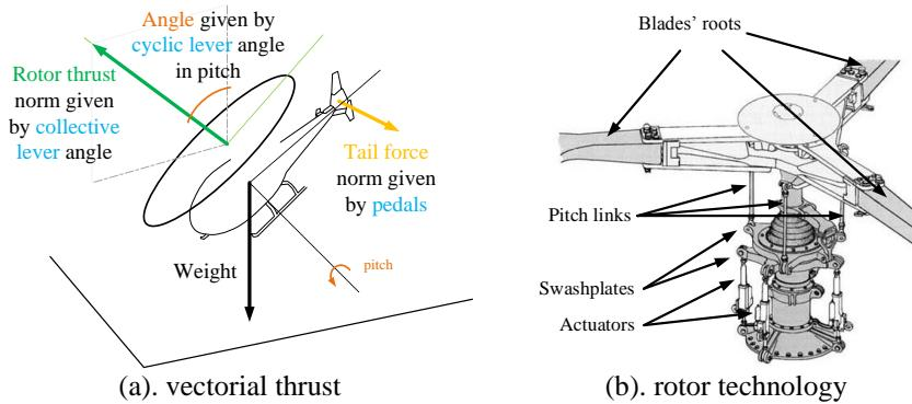
**Figure 1-4. Helicopter main rotor thrust vector and technology**
