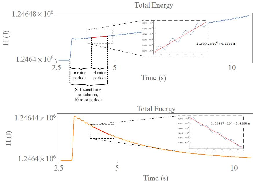
**Figure 5-10. Computation of  $\hat{H}$ , a linear regression of total energy over a few rotor periods**
