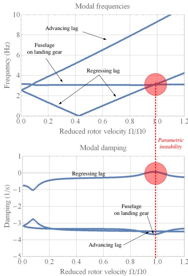
**Fig. 21. Frequency coalescence and regressing lag mode damping loss**
