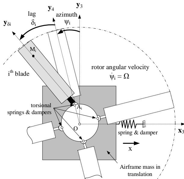
**Figure 5-7. Simplified rotor-airframe model for ground resonance,
