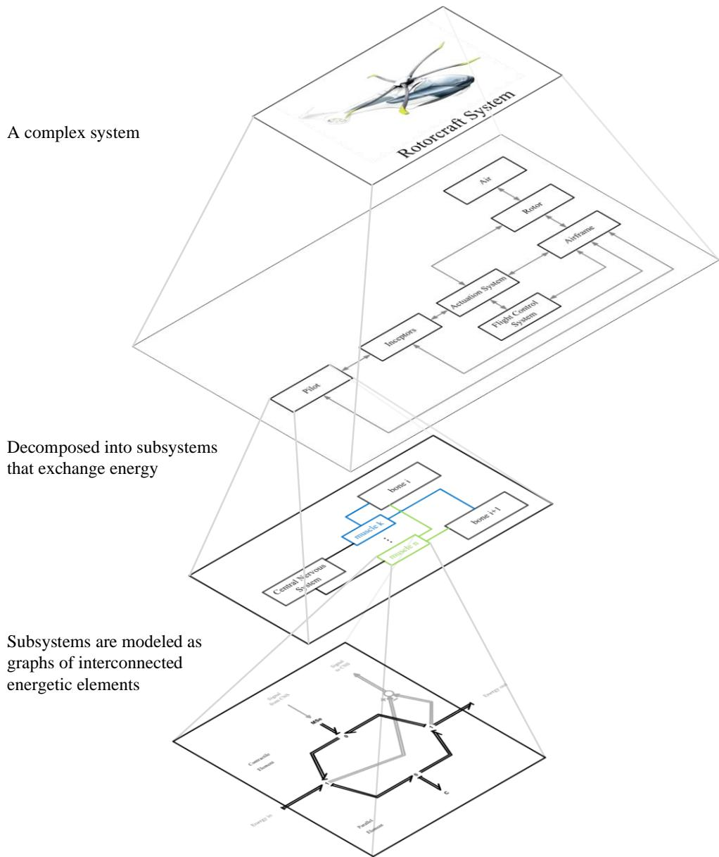
**Figure 1-9. Bond graphs for a systems approach of modeling**
