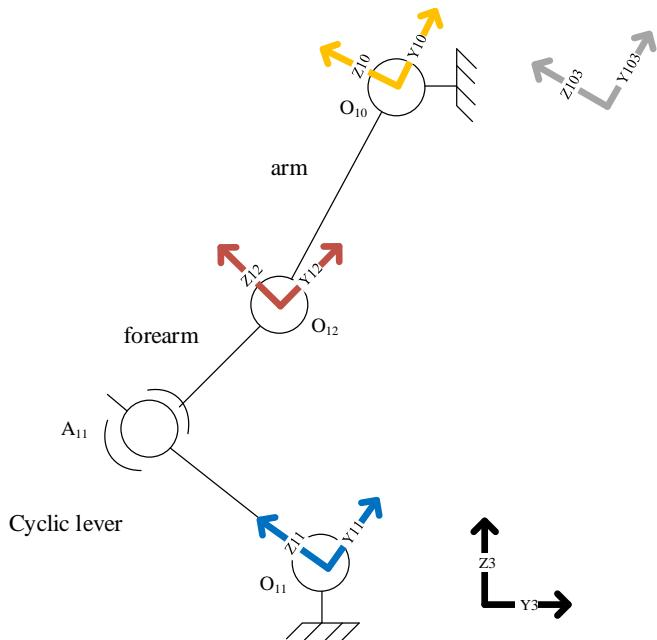
**Fig. 15. Axes definitions of the upper limb multibody system**
