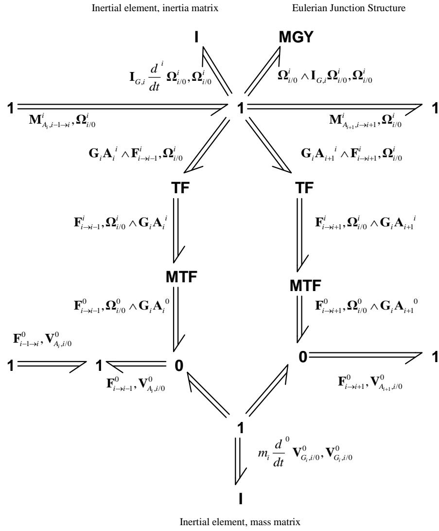
**Figure 2-5. Multibond graph of the  $i^{\text{th}}$  rigid body spatial motion (effort, flow) at each bond**
