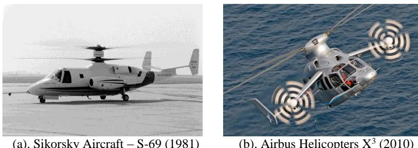
**Figure 1-6. No tail rotor unconventional rotorcraft architectures (photos: Sergeant Lloyd H. Cole, Airbus Helicopters ©)**
