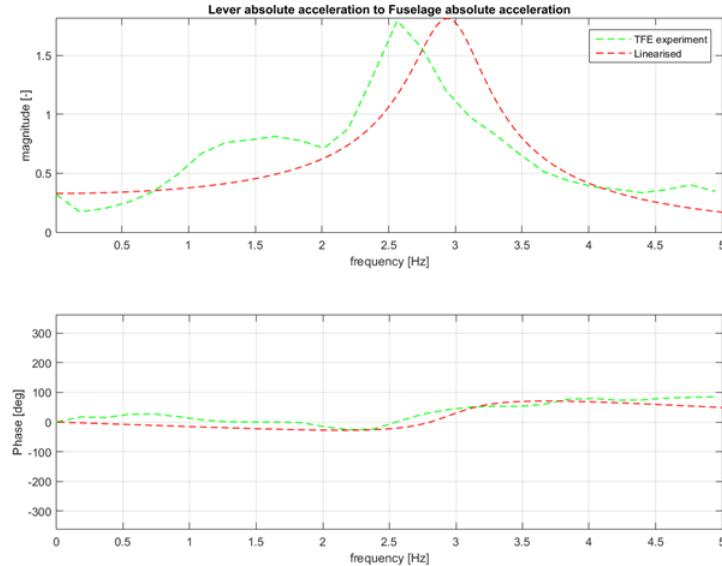
**Figure 2-19. Experiment and numerical identification results of helicopter<sup>13</sup> vertical dynamics**
