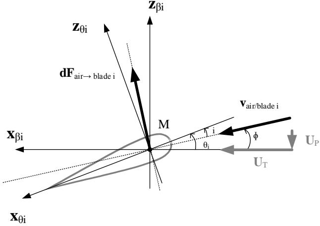
**Figure 2-10. Quasi-steady aerodynamics model – per section**
