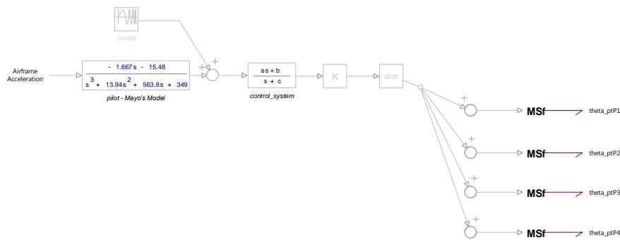
**Figure 2-20. Pilot and control system subsystem model**
