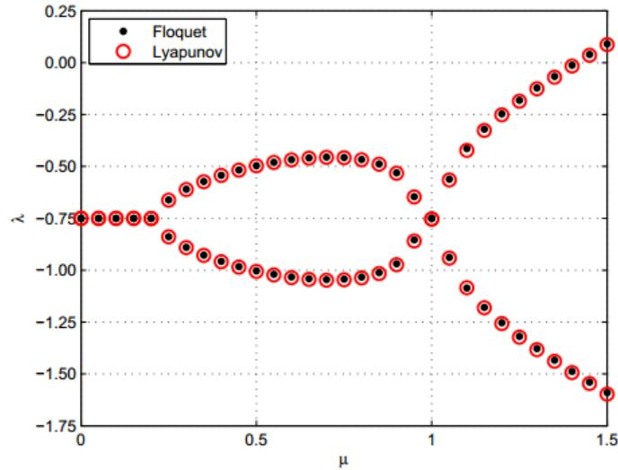
**Figure 5-2. Lyapunov Characteristic Exponents and Floquet multipliers logarithm estimations for varying advancing ratios  $\mu$**
