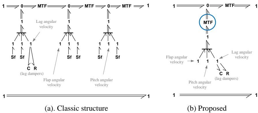
Figure 2-9. Concatenation of three revolute joints proposal
