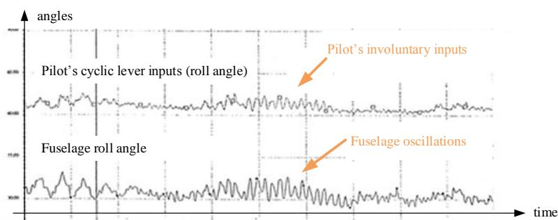
**Figure 1-7. Roll oscillations measured during a flight test**
