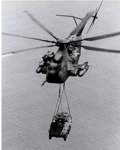
**Figure 3-2. Sikorsky CH-53E Super Stallion with external slung load**
