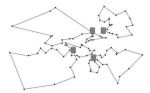
Figure 6: Solution for a medium-size MDVRP with 4 depots (cylinders).
