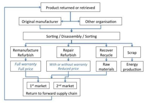
Figure 2: Generic model of reverse supply chains
