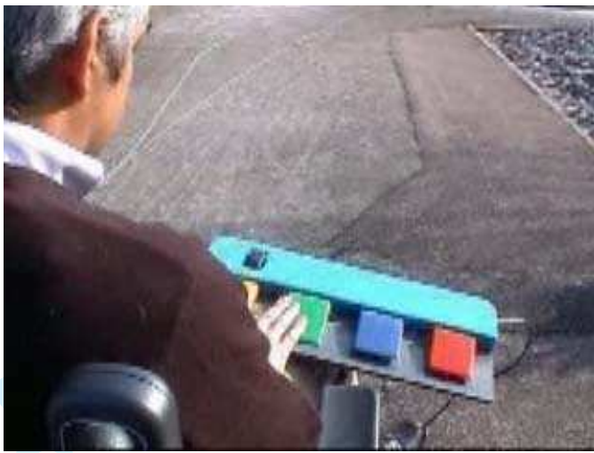
Figure 18 Video still of a driver testing the veer compensating system during an early outside test
