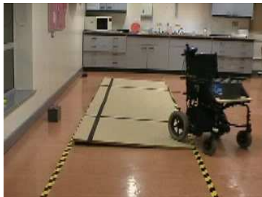
Figure 19 Video stills from an indoor veer test in the laboratory on a 4 meter ramp (with a left slope of 3^\circ ) with only the forward switch control activated.
