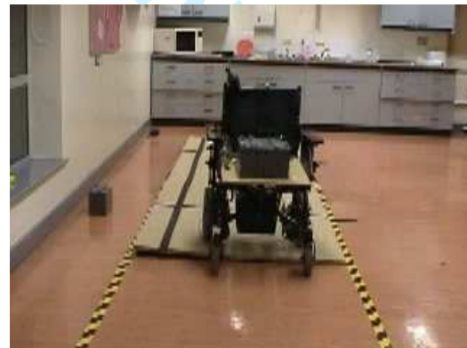
Figure 20 Video stills from an indoor veer test in the laboratory with the forward switch control and sensor system activated.
