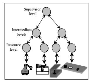
Figure 2. Centralised hierarchical architecture
