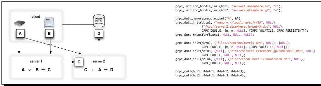
Figure 6.3: Data prefetching example with the GridRPC API.
