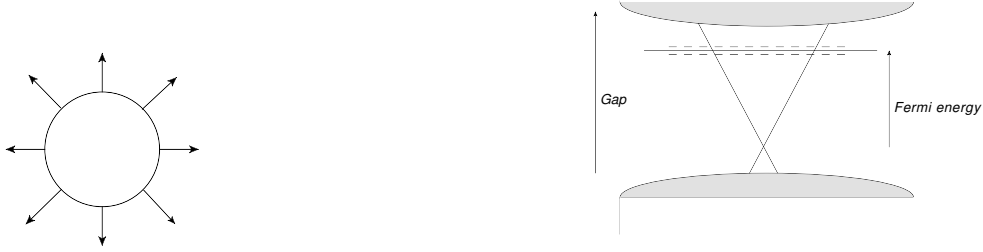
Figure 5.3: Left : projection of the spin for different eigenvectors around the Fermi surface. Right : representation of the different scale of energies in the regime of weak disorder. The dotted line around the Fermi energy line correspond to the states relevant to transport. The energies are counted with respect to the Dirac point.
