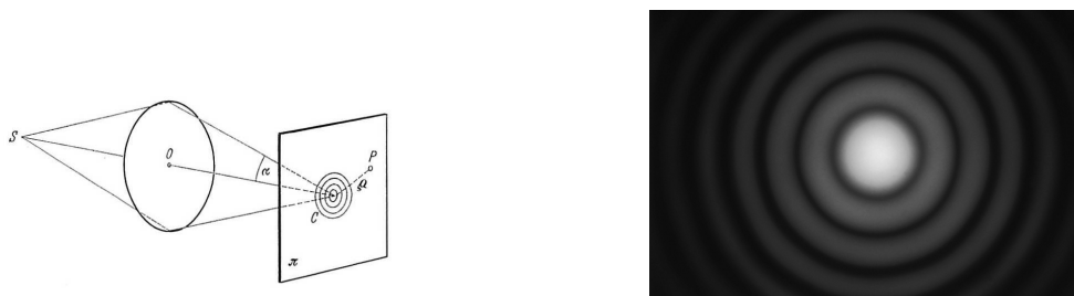
Figure 5.1: Left : principle of the diffraction of the light by a circular hole, right : diffraction pattern observed. Pictures from Atlas de phénomènes d'optiques , Springer-Verlag
