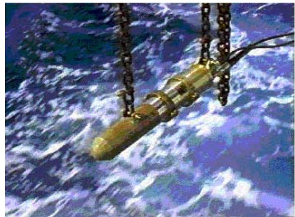
Figure 5: High-pressure seismic air gun
