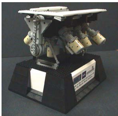
This model of MISR was built out of Lego bricks by the master model-builders at Legoland, California. On Terra, MISR is upside-down from this. MISR's nine cameras are represented with the blocks and wheels sticking out at odd angles. Light enters each camera through holes you can't see here.
